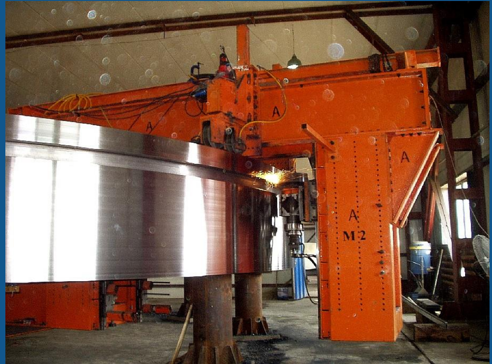
On-Site Machining by Self Leveling Machines (SLM)
